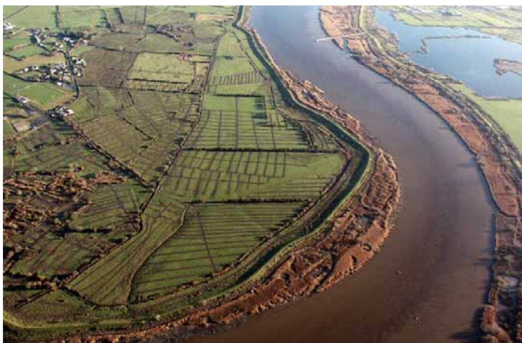
Illus. 5—Aerial view of the Shannon estuary looking east towards Limerick, at the point where the ring road will tunnel beneath the Shannon. The estuary is now contained by flood banks with only narrow reed beds on either side (brown in photo). Former tidal saltmarshes, now reclaimed, occupy most of the photo. The houses on the left are built on a low 'island' at Coonagh, rising just above the marshes. Bunlicky Lake, to the right of the Shannon, is a flooded quarry where the alluvium was dug for cement manufacture (TVAS [Ireland] Ltd)
