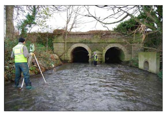
Plate 9: Working-shot of Total Station survey undertaken along upstream side of Balheary Bridge (Feature 3), Ward River.
