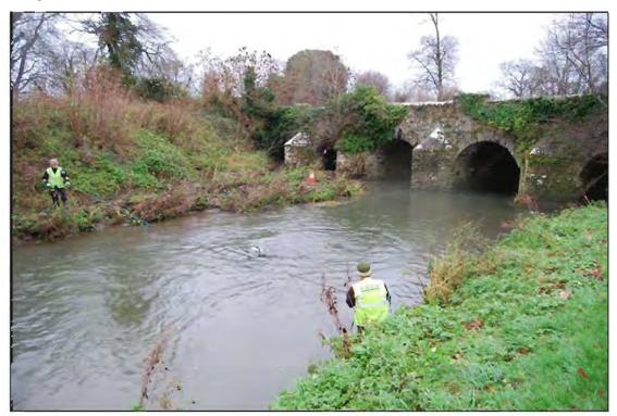
**Plate 4:** Working-shot of diver undertaking riverbed survey along upstream side of Lissenhall Bridge, Broadmeadow River. Note: diver tethered to counteract against river-flow.
