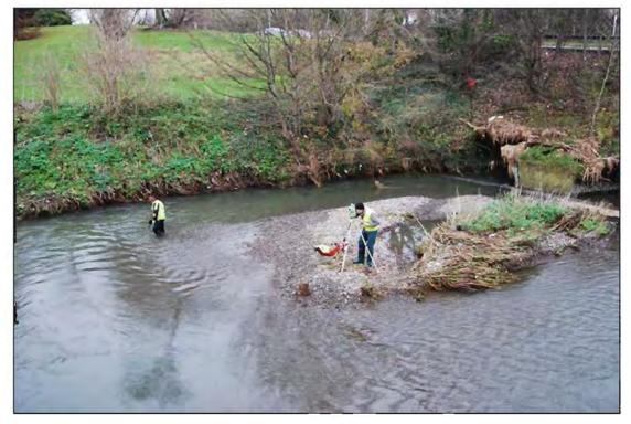
Plate 8: Working-shot of metal-detector survey and Total Station survey undertaken along downstream side of Lissenhall Bridge (Feature 1), Broadmeadow River.
