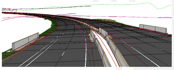
Geometric cross section optimised to maximise sight distance
