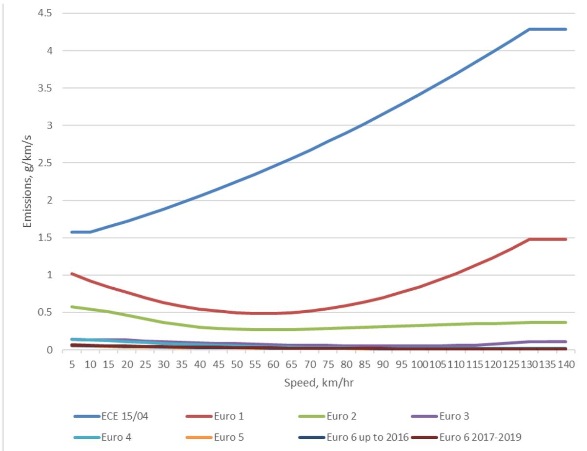
Figure G1 Speed / Emission Profile for Medium Petrol Cars
