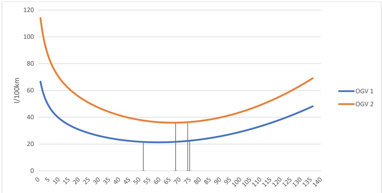
Figure F2 TUBA Fuel Consumption vs Speed Profiles for HDV
