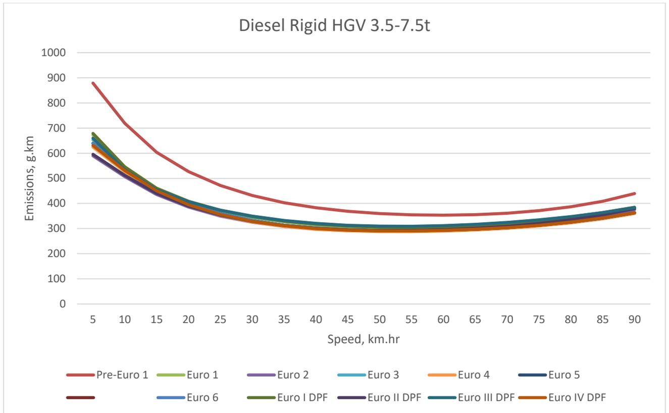
Figure F6 CO<sub>2</sub> Emissions, Rigid Diesels 3.5-7.5t
