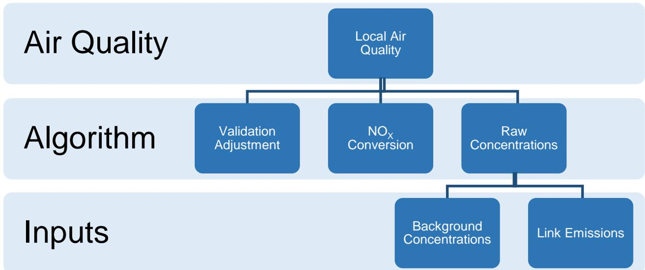
Figure 1.2 Modular Approach Schematic to Air Quality Calculations
