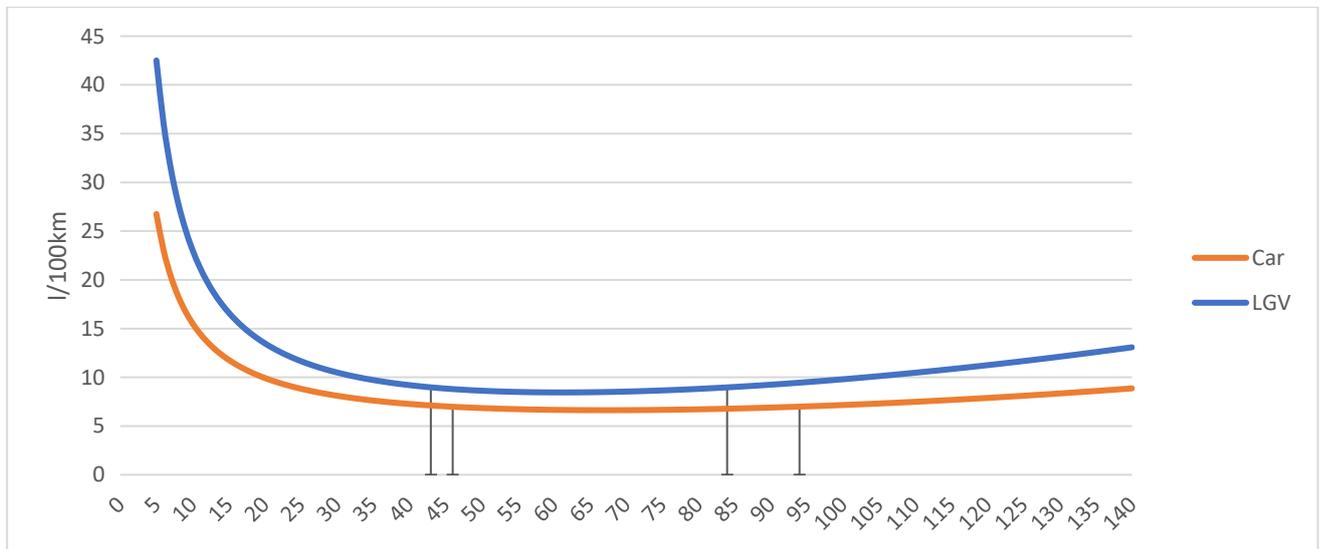
**Figure F1 TUBA Fuel Consumption vs Speed Profiles for LDV**
