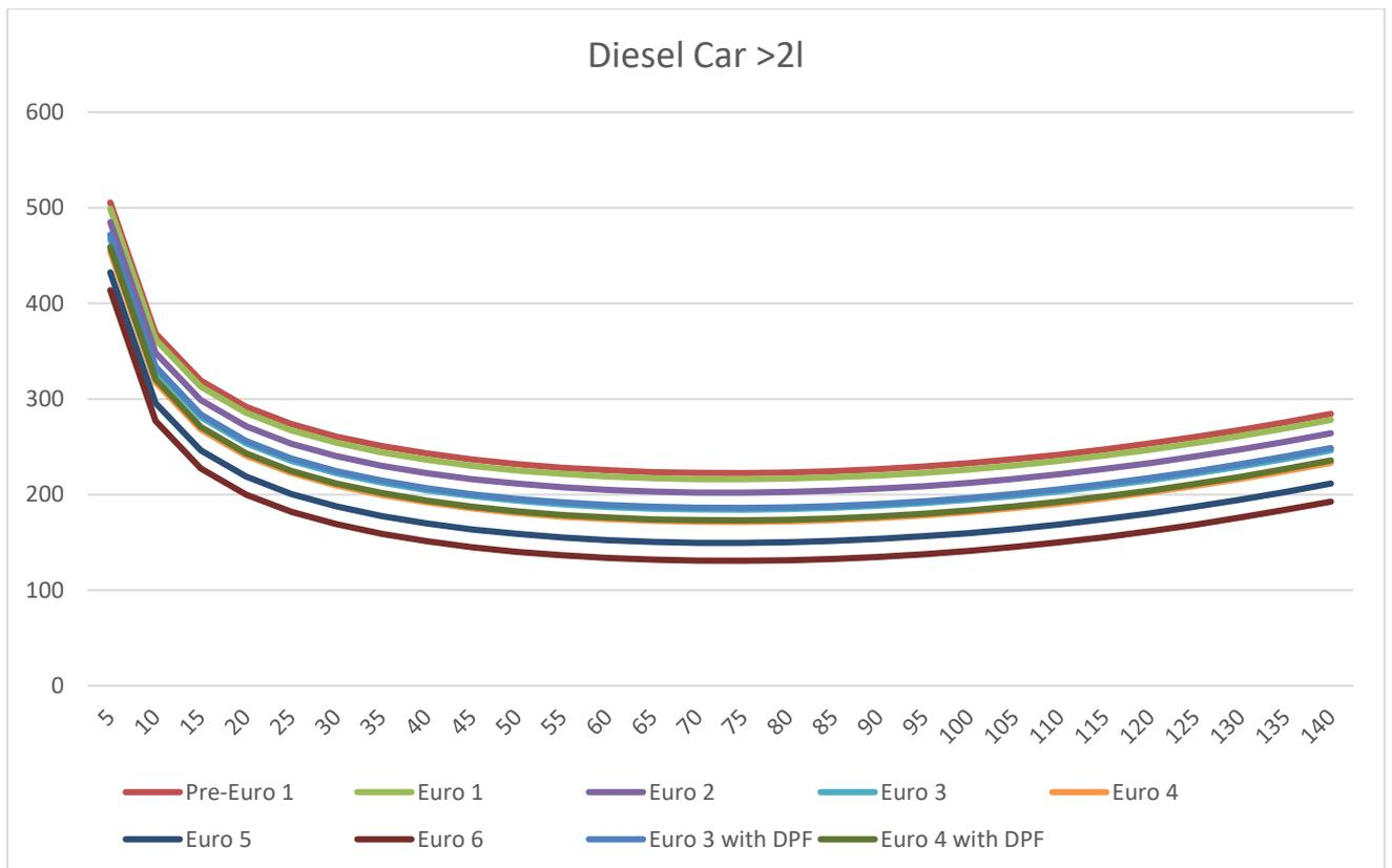
**Figure F5 CO<sub>2</sub> Emissions, Large Diesel Cars**
