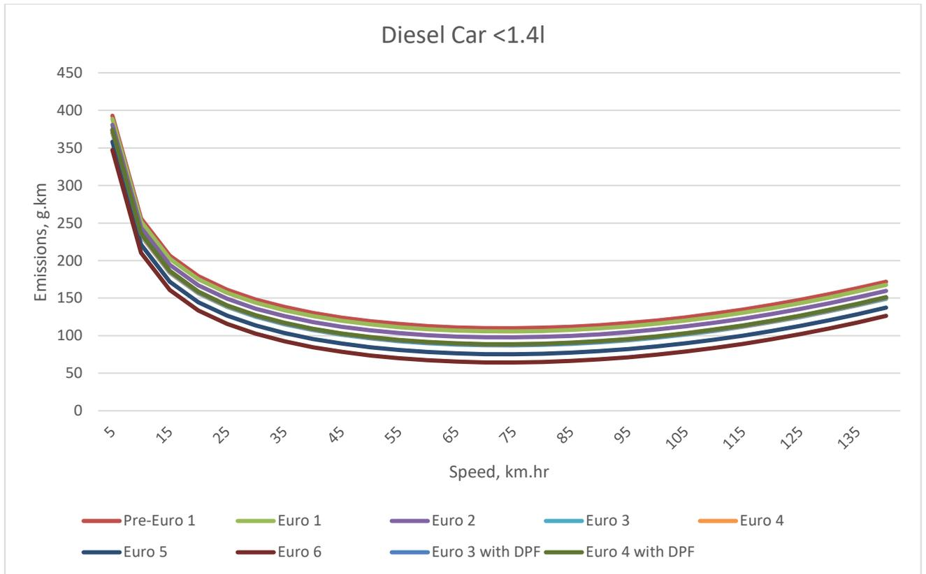
**Figure F5 CO<sub>2</sub> Emissions, Small Diesel Cars**
