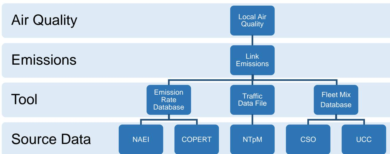
Figure 1.1 Schematic of the TII REM and Source Data
