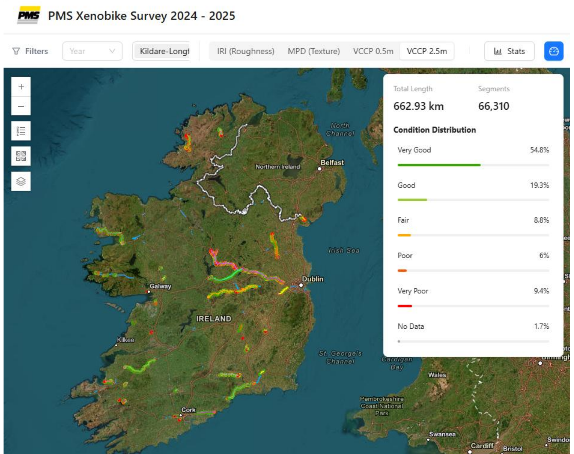
Figure 8 – PMS Web map displaying ATI pavement Condition
