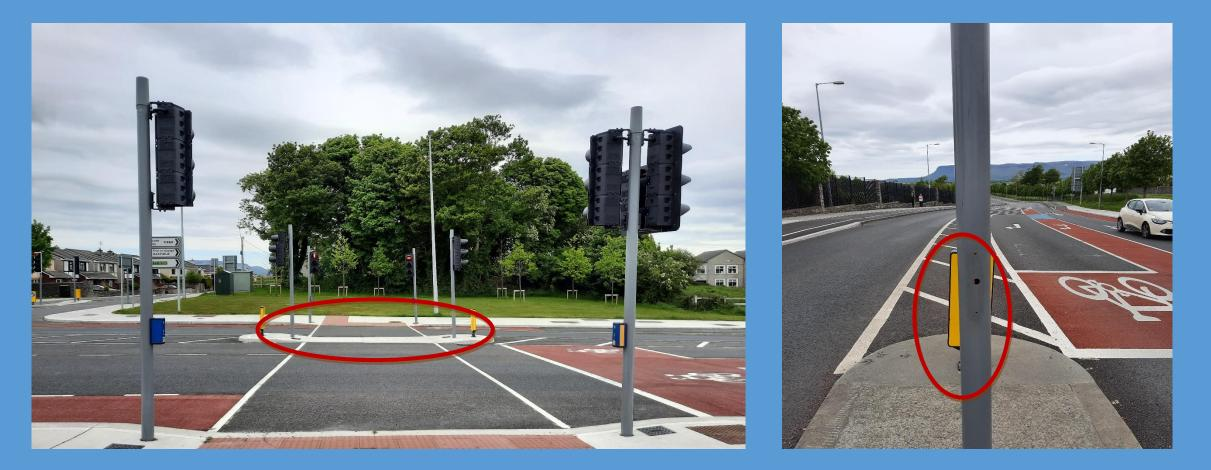
Signalized Crossings problems Traffic focused staging No detection - expect to cross in predetermined time within phase Trapped Pedestrians in central island
