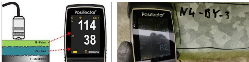
Figure 3.4 – (Left) Illustration of Positector Probe; (Right) Test area markings and Positector Probe results
