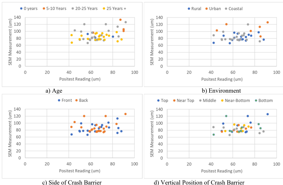
Figure 11: Data from previous graph ( Figure 10 ) broken down by a) Age, b) Environment, c) Side and d) Vertical Position of Crash Barrier. For clarity, the error bars were removed.
