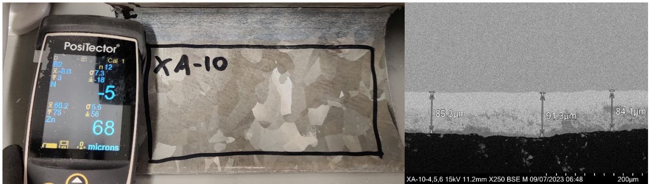
Figure 19: Photograph of front area of N55-LK-RN80 (XA-10) (left) and correspond SEM image (right). Galvanised zinc coating has been measured at 12 points using the Positector and 9 points via SEM.
