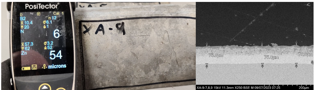
Figure 18: Photograph of front area of N55-LK-RN80 (XA-9) (left) and correspond SEM image (right). Galvanised zinc coating has been measured at 12 points using the Positector and 9 points via SEM.
