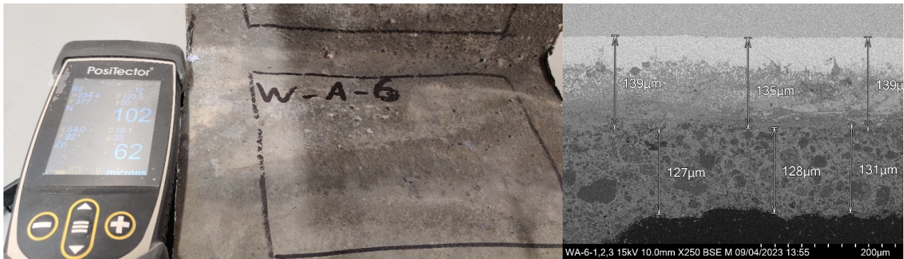
Figure 16: Photograph of front area of N55-ATH (WA-6) (left) and correspond SEM image (right). Galvanised zinc coating has been measured at 12 points using the Positector and 9 points via SEM.
