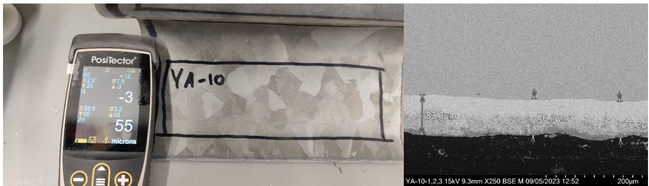
Figure 21: Photograph of front area of N59-GY-SB09A (YA-10) (left) and correspond SEM image (right). Galvanised zinc coating has been measured at three points.
