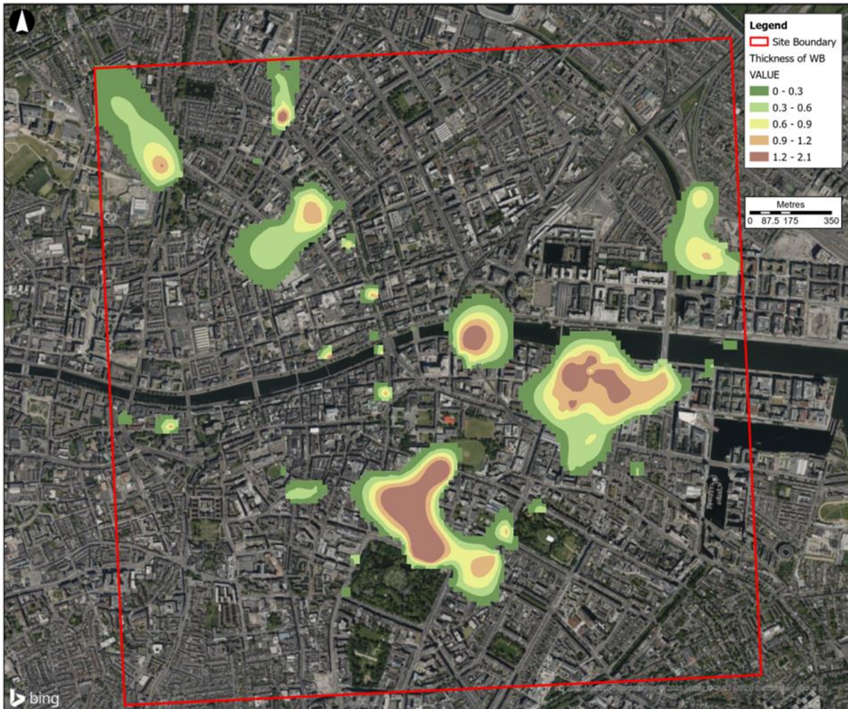
Figure 32 Thickness of weathered bedrock generated in Leapfrog geological modelling software.
