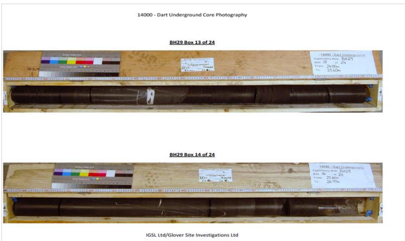
Figure 54 Core photograph of DART Underground BH29 showing aperture range from open to wide (0.05m to 0.10m spacing) without infilling
