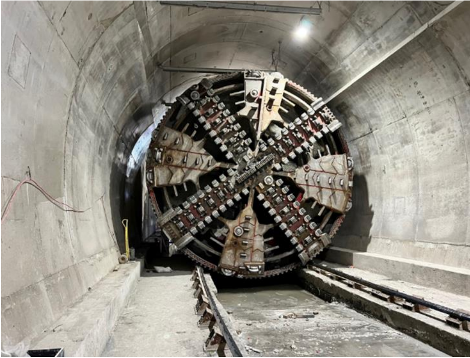
Figure 112 TBM Cutter Head used in New Zealand's City Rail Link in Auckland (City Rail Link, 2022).
