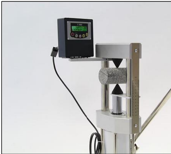
Figure 22 Diametrical PLT ( https://www.geotech.hr/en/point-load-test-plt/ ).
