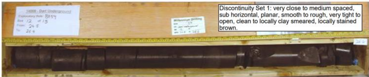
Figure 51 Typical discontinuity spacing (BH54; DART Underground)
