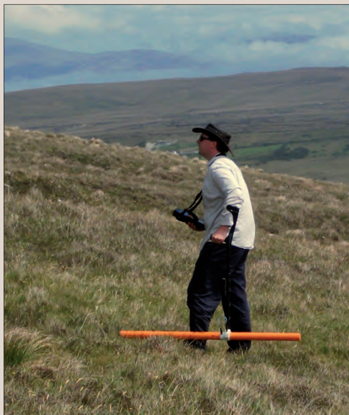
The latest technology—in this case a new electromagnetic device—being used by the author to assess its suitability for road schemes. (Image: NRA Fellowship Programme, University of Bradford)
