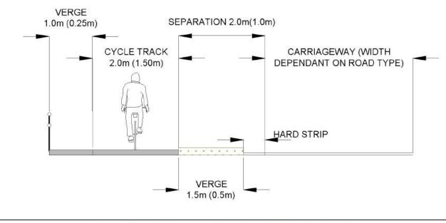
Figure 4.2: Off-Road One-Way Cycle Track (Low Volume)
